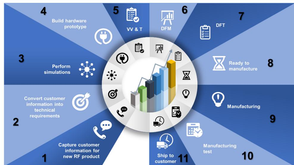
**Figure 1.** RF electronic product design and manufacturing process life cycle.
