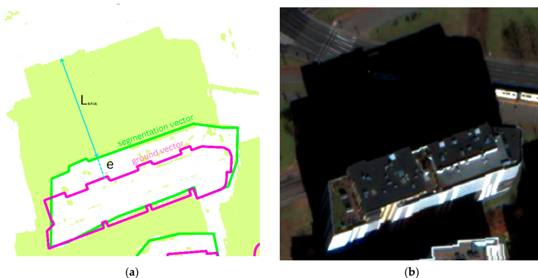
Figure 4. (a) Shadow length estimation—segmentation vector (green) versus ground vector (purple); light green color represents shadow. (b) Imagery fragment corresponding to (a).
