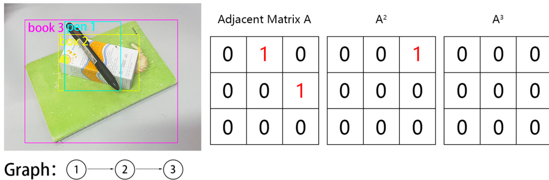
Figure 2. The left-hand side of the figure presents a stack of objects and its directed graph, while the right-hand side shows the corresponding adjacency matrix and its power. To calculate the secure grasping, we utilize the n -th power of the adjacency matrix. Elements of the matrix's i -th row and j -th column denote the probability of covering.
