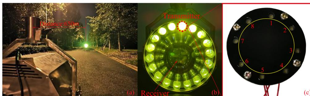
**Figure 11.** (a) Test scenario; (b) the full-duplex dual-channel FSO communication system; (c) the smallest transmitting unit.
