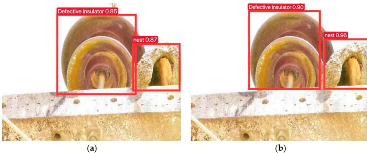
**Figure 8.** Model training before and after enriching the dataset for the detection results of defective insulators: (a) before enriching the dataset; (b) after enriching the dataset.
