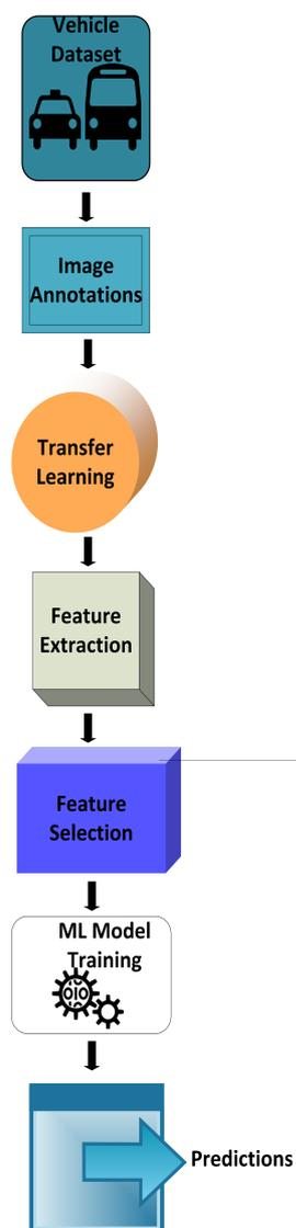
Figure 1. Proposed vehicle make and model recognition system.
