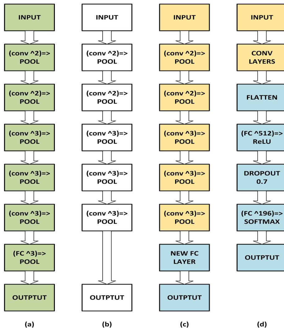
**Figure 2.** CNN architecture for transfer learning. (a) original CNN. (b) Our network without the FC layer. (c) Tuned network head without updating the base weights. (d) Fine-tuning of the FC layer head and the final CONV block.
