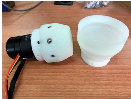
**Figure 2.** A pair of cam-ball-type connectors. Active connector on the left and passive connector on the right.
