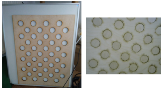
Figure 5. Plywood thermal calibration board.
