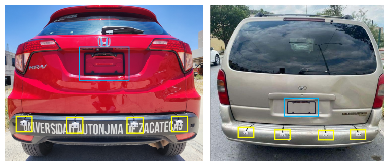
Figure 3. Experimental setup. The blue box = reverse camera installed, yellow boxes = ultrasonic sensors.
