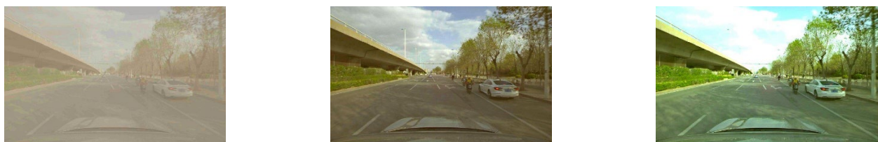
Figure 14. The combination of the dark channel prior algorithm and Strategy 3. Images with a high concentration, medium concentration, and low concentration are reduced by 256 times via bilinear interpolation, to improve the processing efficiency for fogged images. After dark channel defogging, the images with fog removed are upsampled 4 times, and the images are expanded to 256 times the original size. Gaussian transformation is then applied to the images.
