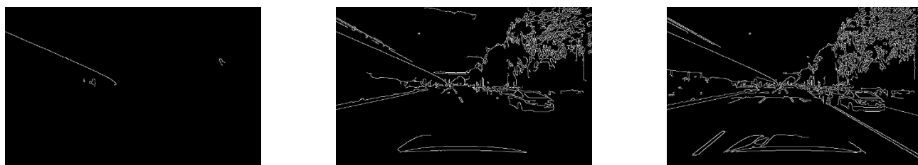
Figure 20. The results obtained via the canny algorithm on the defogging pictures in high-concentration fog, defogging pictures in medium-concentration fog, and defogging pictures in low-concentration fog, obtained via the original dark channel prior defogging algorithm.
