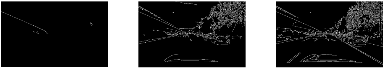
Figure 22. The results obtained via the canny algorithm for the defogging picture for a high-concentration fog day, the defogging picture for a medium-concentration fog day, and the defogging picture for a low-concentration fog day, obtained via Optimization Strategy 3 (referring to the fusion of dark channel prior and Optimization Strategy 3).
