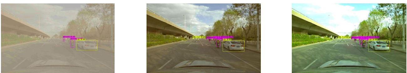
Figure 32. YOLOv5, respectively, detects vehicles and pedestrians in defogging pictures with high-concentration fog, medium-concentration fog, and low-concentration fog.
