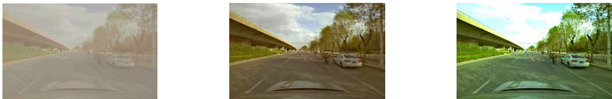
Figure 13. The combination of the dark channel prior algorithm and Strategy 2. Images with a high concentration, medium concentration, and low concentration of fog are reduced by 256 times after Gaussian transformation and 4-time downsampling processing, which improves the processing efficiency for foggy images. The picture is obtained via bilinear interpolation, to enlarge the picture 256 times after the fog removal.
