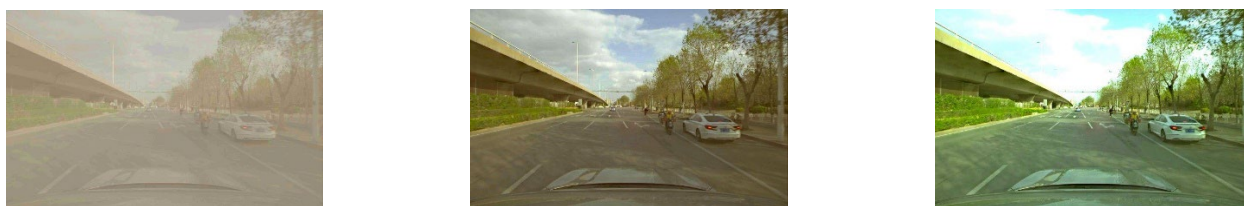
Figure 15. The combination of the dark channel prior algorithm and Strategy 4. Images with a high concentration, medium concentration, and low concentration of fog are reduced by 256 times through bilinear interpolation, to improve the processing efficiency for foggy images. After the dark channel is defogged, images with defogging are reconstructed via bilinear interpolation, and the defogged images are enlarged by 256 times.
