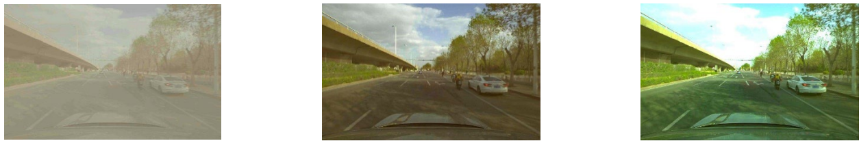
Figure 16. The pictures with high-concentration fog, medium-concentration fog, and low-concentration fog, after the original dark channel defogging algorithm.
