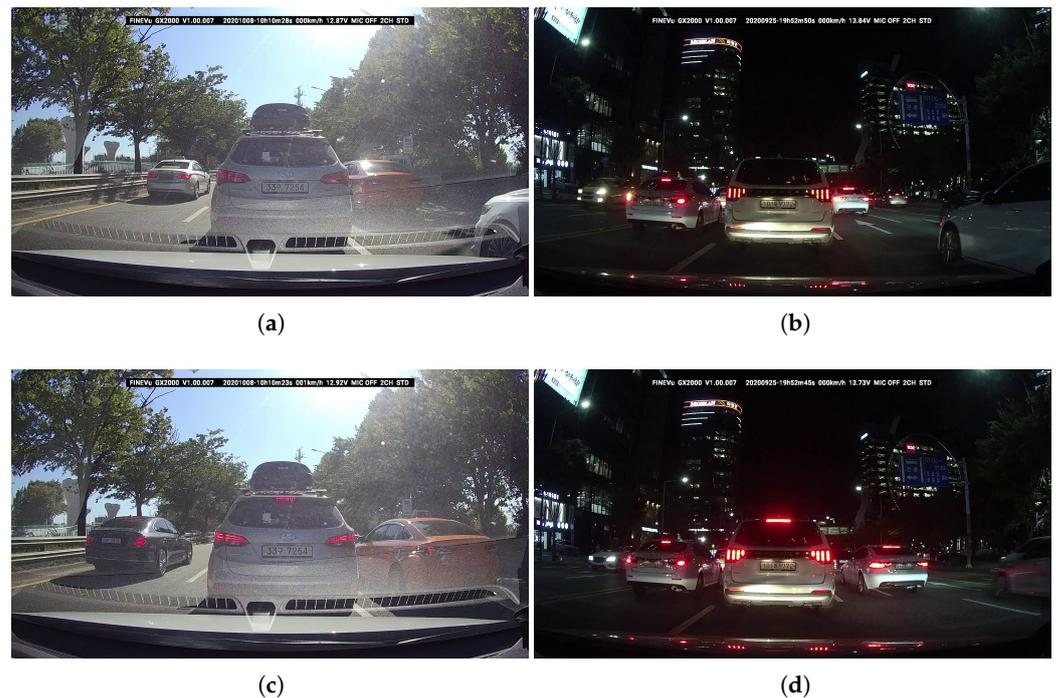
**Figure 2.** Illustrative cases in which it is difficult to determine the operation of brake lights based on single image. (a) Light reflection from LED lights. (b) Confusion with tail lights. (c) Preceding image of (a). (d) Preceding image of (b).
