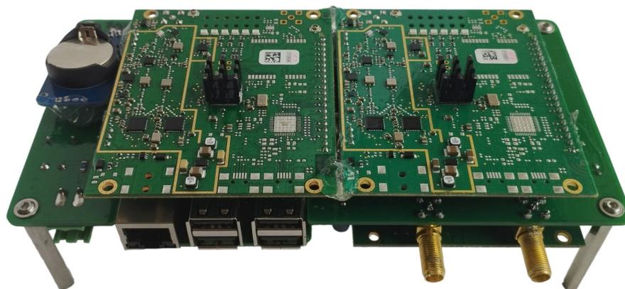
**Figure 3.** Photo of the LoRaWAN sniffer internal hardware.
