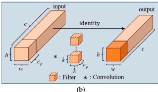
**Figure 5.** Comparison of DWConv and PConv. (a) Structure diagram of deep convolution; (b) structure diagram of partial convolution.
