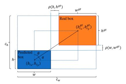
**Figure 3.** Schematic diagram of the parameters of the loss function.
