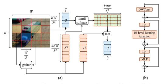
Figure 4. (a) Structure of the Bi-Level Routing Attention; (b) Structure of the Biformer block.
