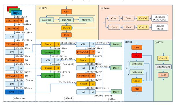
**Figure 1.** The network structure of YOLOv8. The w (width) and r (ratio) in Figure 1 are parameters used to represent the size of the feature map. The size of the model can be controlled by setting the values of w and r to meet the needs of different application scenarios.
