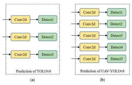
Figure 7. (a) Detection head of YOLOv8; (b) detection head of our proposed method.
