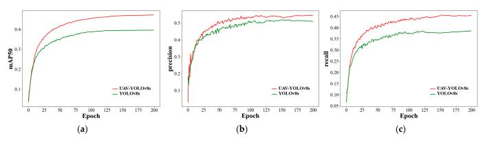
**Figure 10.** (a) Training curve of UAV-YOLOv8s and YOLOv8s in mAP; (b) training curve of UAV-YOLOv8s and YOLOv8s in precision; (c) training curve of UAV-YOLOv8s and YOLOv8s in recall.
