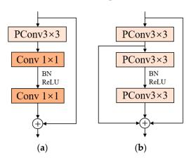
**Figure 6.** Comparison of FasterNet block and Focal FasterNet block. (a) Structure diagram of FasterNet block; (b) structure diagram of our proposed module.
