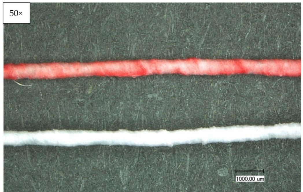
**Figure 7.** Optical characterization of the temperature sensing heating yarn with color change; **top:** normal condition, **bottom:** heated condition.
