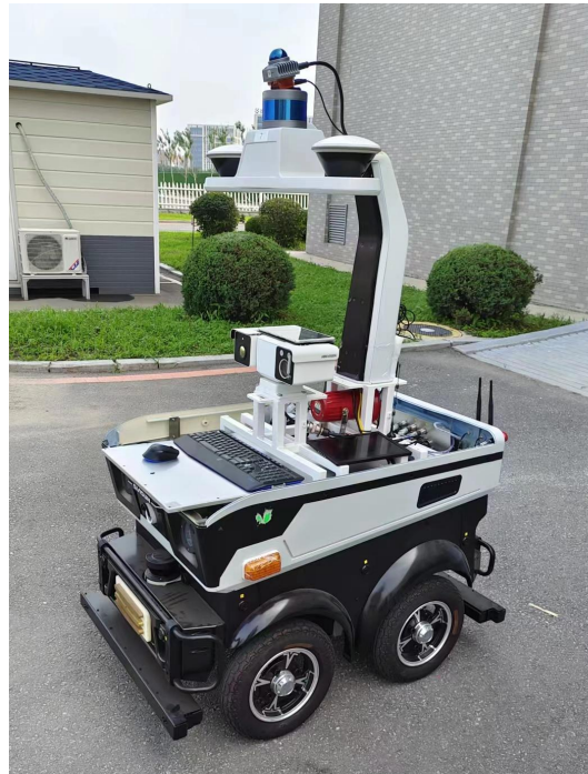
Figure 4. The UGV for collecting indoor and outdoor datasets.
