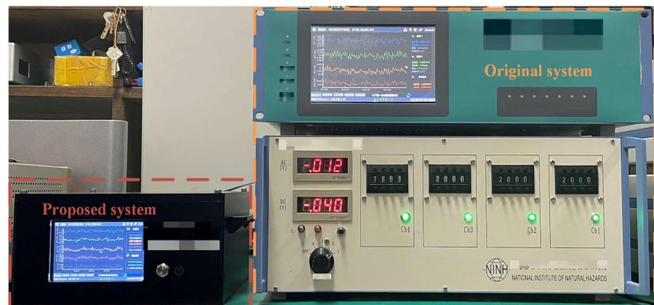
**Figure 9.** Comparison of the original system and the FPGA-based observation system.
