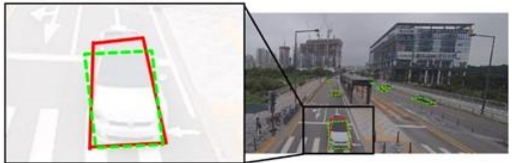
Figure 15. The limitations of the parallelogram assumption of the PSA-based approach. The red and the green dashed quadrilaterals represent the ground truth and the detected BFQs, respectively.
