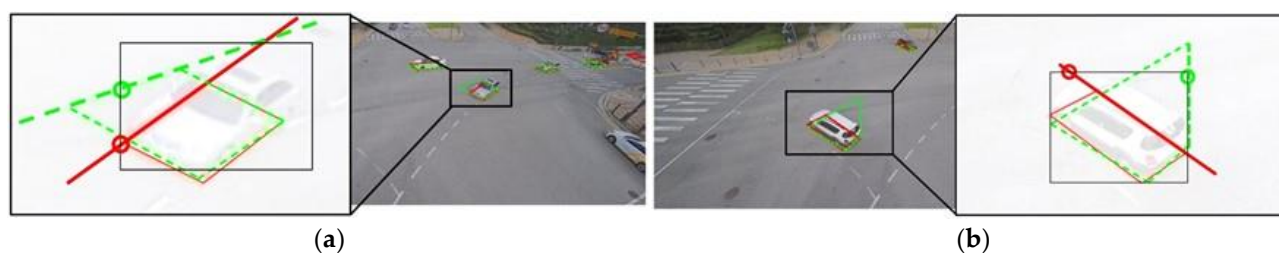
Figure 19. The BFQs resulting from the intersection point with the errors in the predicted ratio. The red circle, line, and quadrilateral are the intersection point, the extended line of an edge, and the BFQ of the ground truth, respectively. The green circle, line, and quadrilateral are the same as the detected BFQ. The bounding box is shown as the black rectangle: (a) result of the L2 method; and (b) result of the L3 method.
