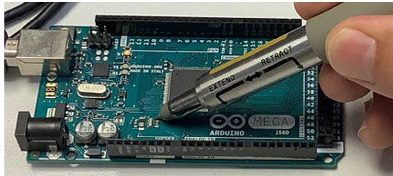
**Figure 6.** High-impedance probe measurement of the actual frequency of the ceramic oscillator.
