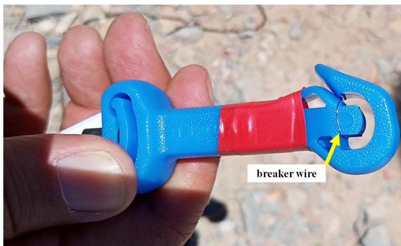
Figure 14. Surface detonator with 1x ø 0.19 mm copper break wire.
