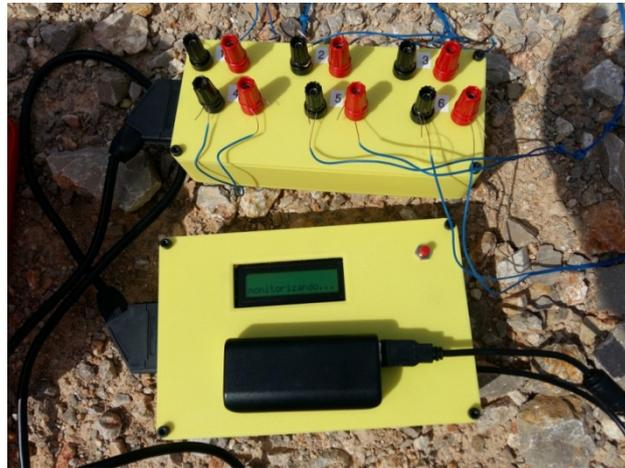
**Figure 2.** Equipment built. Quick connection box (**upper part**) and microcontroller casing (**lower part**).
