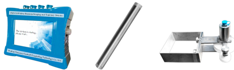
Figure 2. ZKXG100 mine-drilling imaging trajectory detection device; left: host; middle: 24 mm sensor; right: depth detector.
