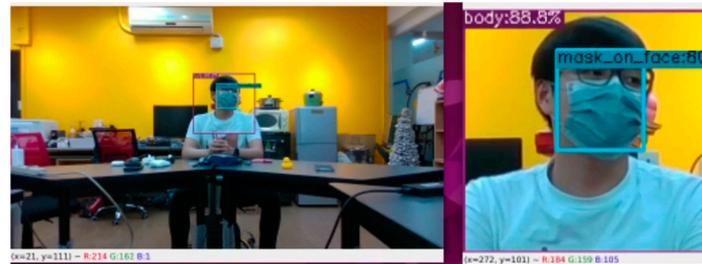
**Figure 5.** Sound source positioning-assisted filtering after YOLO person detection (left) and the output low-confidence masked target person (right).
