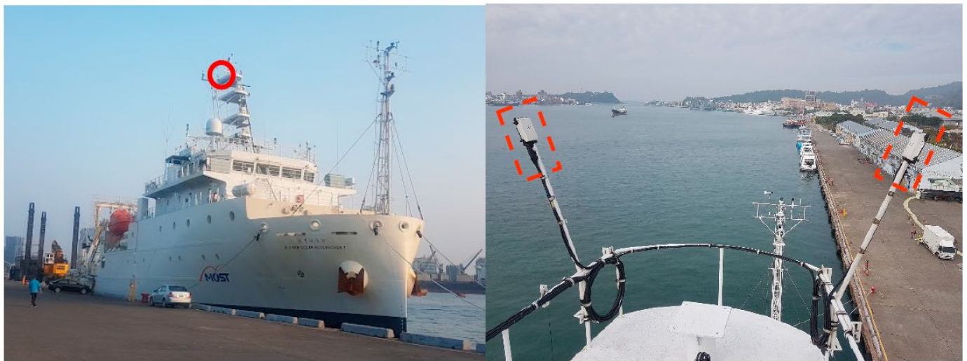
Figure 3. The (left panel) shows a picture of the R/V NOR1, where the red circle indicates the positions of two GPS&SBAS receiving antennas. The (right panel) shows the two GPS&SBAS-R receiving antenna installations by dotted red rectangles.
