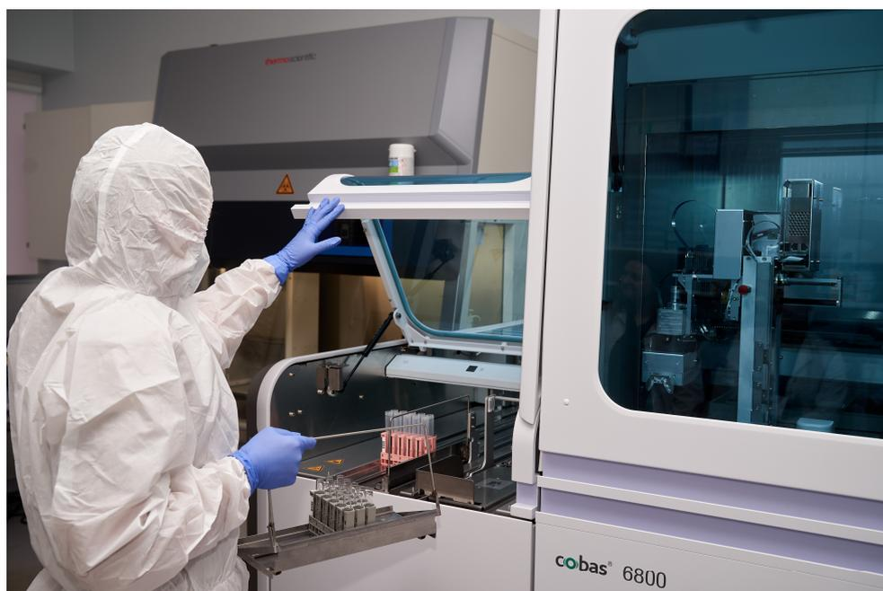
**Figure 4.** Procedure of Cobas<sup>®</sup> PCR Media containing virus (positive samples) placement to the Cobas<sup>®</sup> 6800 system after irradiation.
