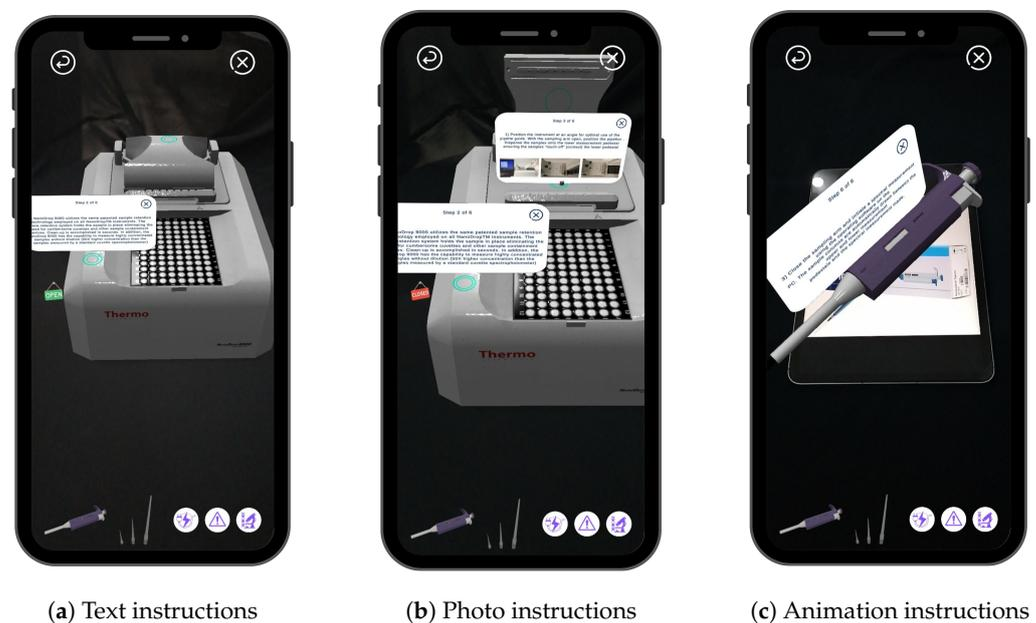
**Figure 3.** The application generated an exploded view of the NanoDrop Spectrophotometer, which highlights its subparts and aids in step-by-step training for operating the machine.
