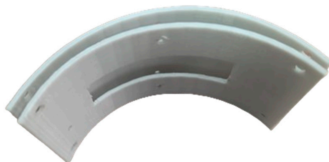
Figure 13. The special mold for the flexible phased array.
