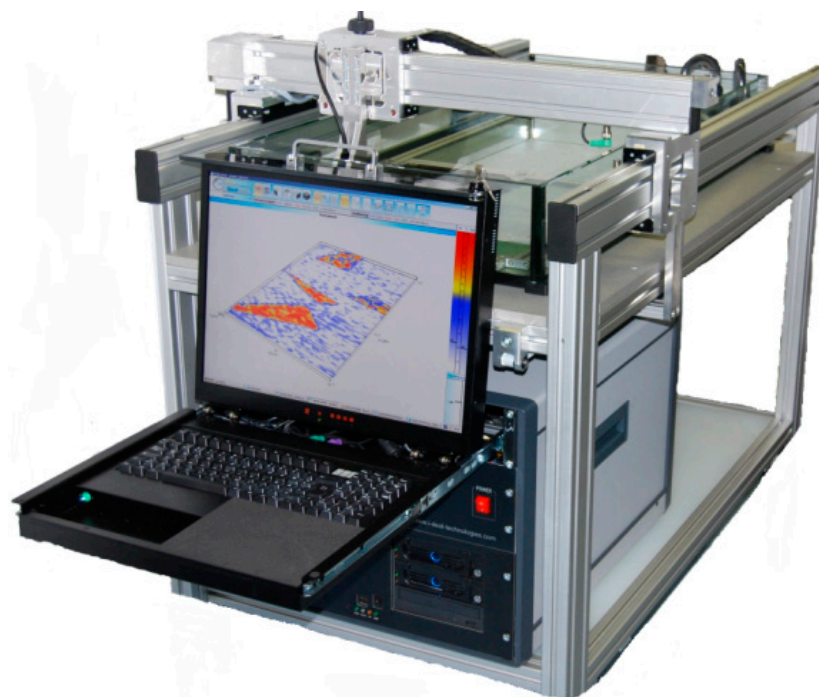
Figure 12. Multichannel ultrasonic inspection system: Idealsystem.
