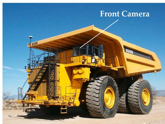
Figure 5. Data collection platform and the position of front camera.
