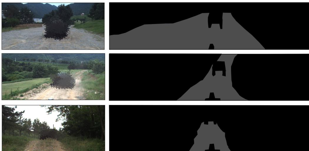
**Figure 9.** The range image, converted from a raw 3D point cloud, was annotated pixel-wise to distinguish between traversable and non-traversable regions. The images on the left show the actual environment of the rough terrain, while those on the right represent the annotation results for the traversable regions.
