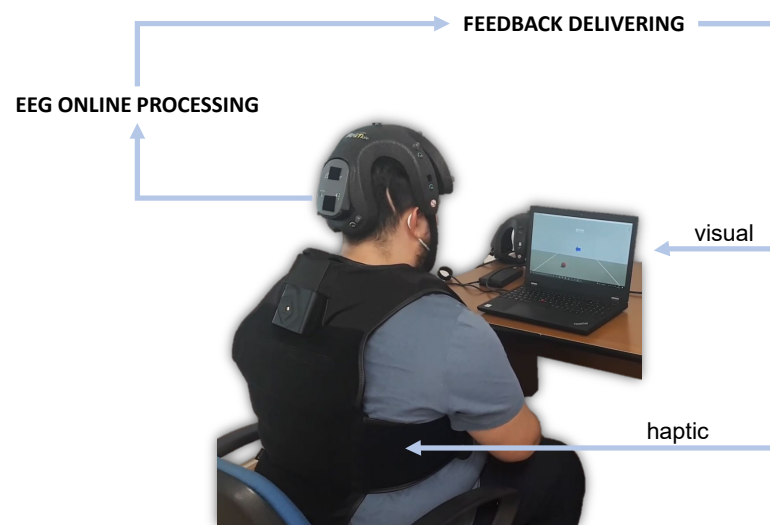
Figure 1. A subject using the proposed BCI system with neurofeedback in extended reality. The system involves EEG acquisition with the Helmate device, online processing, and actuators for visual–haptic feedback delivery.
