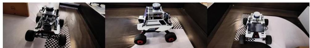
**Figure 32.** A mobile robot with LIDAR used in the experiment.
