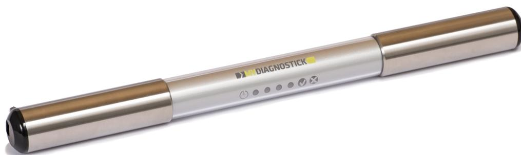
**Figure 1.** The MyDiagnostick device used in our study. The device incorporates two metal handle electrodes and performs an Einthoven I-lead ECG when held by the user.
