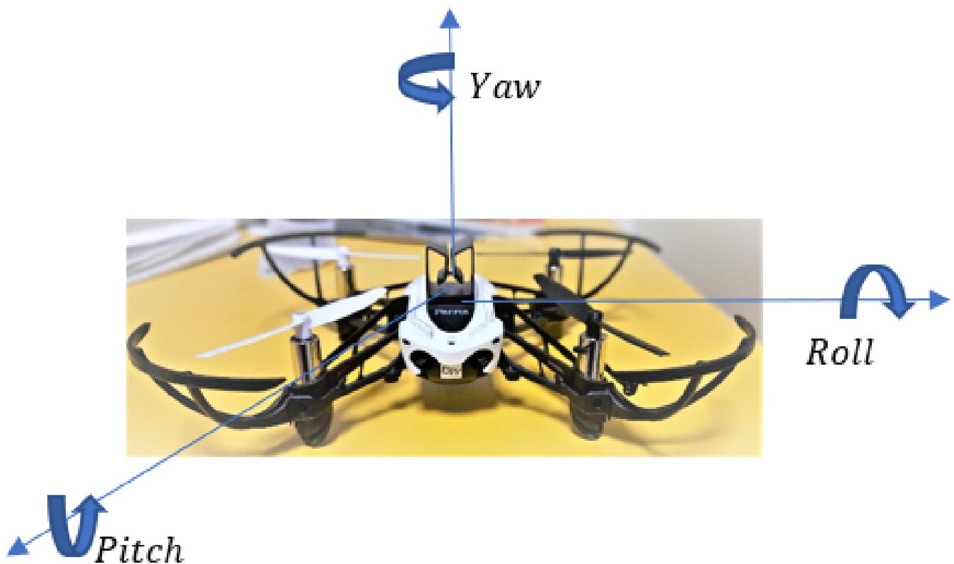
**Figure 1.** Orientation angles of UAV.
