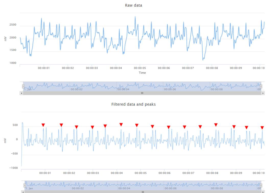
**Figure 5.** Comparison of raw (top) and filtered (bottom) signal under moderate motion conditions.
