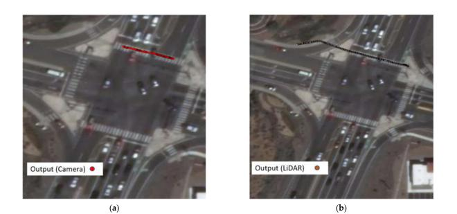
**Figure 17.** (**a**) Sample pedestrian trajectories captured by camera; (**b**) sample pedestrian trajectories captured by LiDAR.
