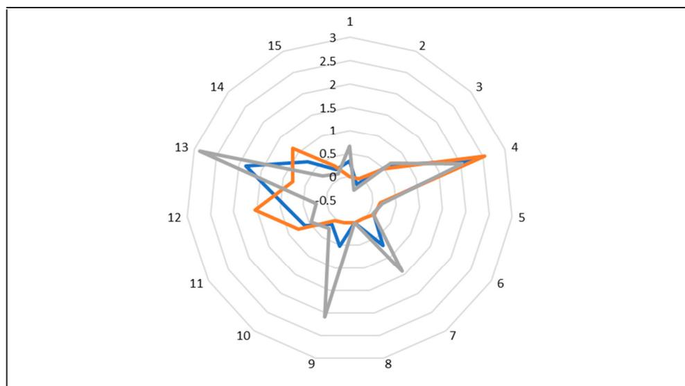
**Figure 8.** The scent pattern of toluene at 2 ppm acquired on three different days. The differences of the individual patterns illustrate the limited reproducibility.
