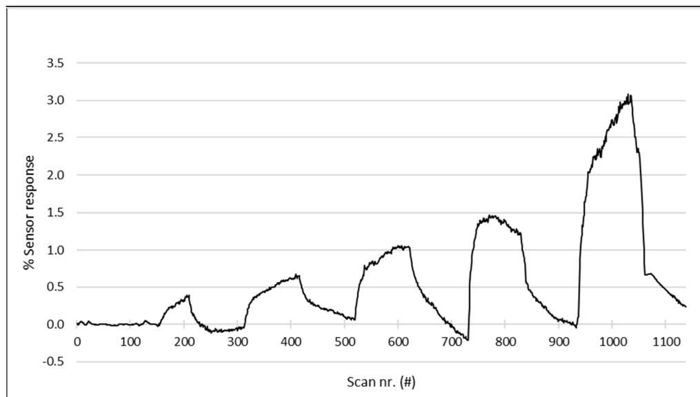
**Figure 3.** The response of the sensor with most sensitive signal for toluene vapor. The concentrations tested are from left to right, 0.5, 1.0, 2.0, 4.0, and 8.0 ppm. The lowest concentration of 0.5 ppm is still visible, and the peak height (% Sensor response) seems to increase by a factor of 2 in every next peak.
