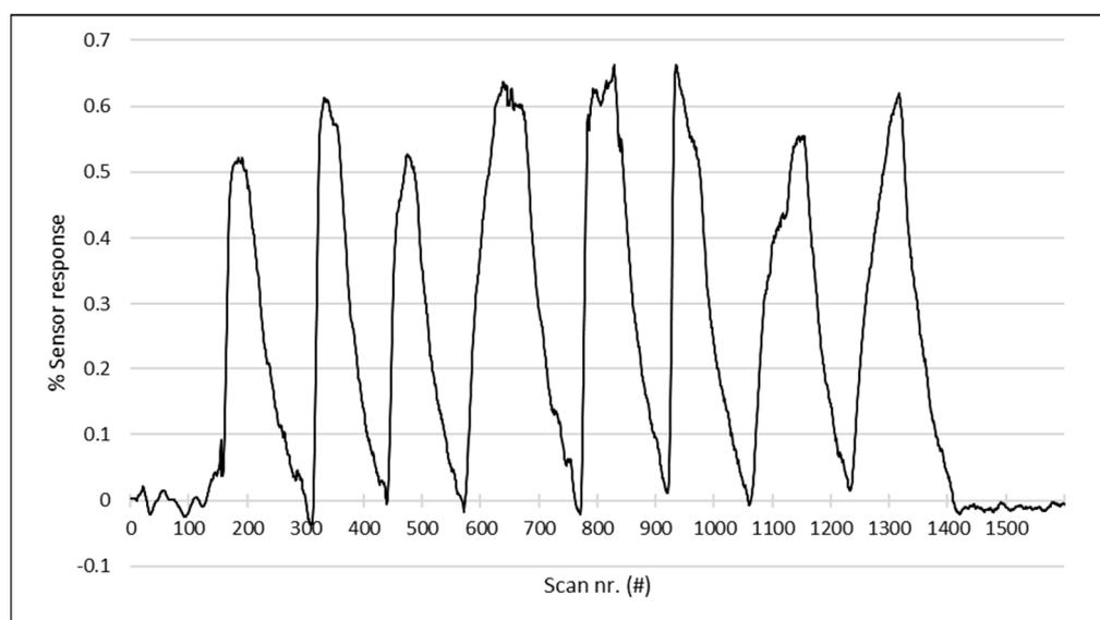
**Figure 5.** Repeatability determined by seven measurements of 2 ppm toluene on the same day.
