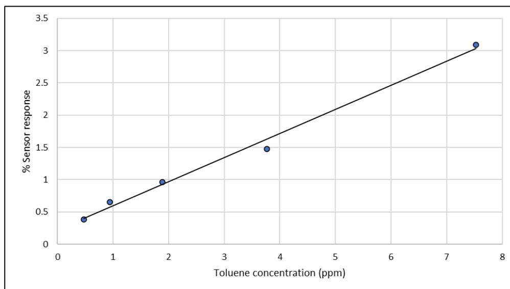
**Figure 4.** Calibration line for toluene concentrations in the range of 0.5–8.0 ppm. The correlation coefficient ( $R^2 = 0.993$ ) indicates that the response is linear in this range.
