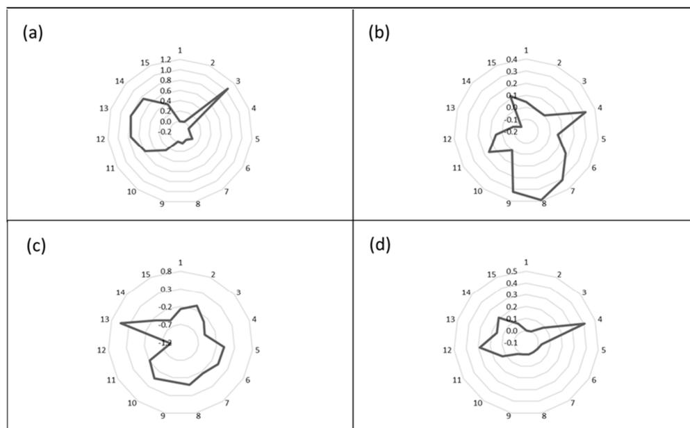
**Figure 2.** Radar plots of the four VOCs ((a); methylamine, (b); acetonitrile, (c); ethyl acetate, (d); toluene) showing clear differences in the image allowing identification of the individual VOCs.
