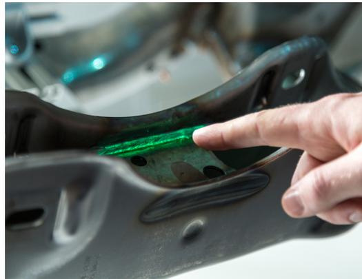
**Figure 5.** The projector highlights a weld on the original metal workpiece.
