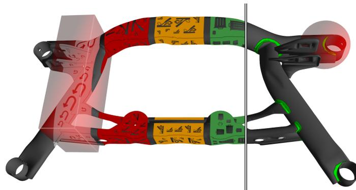
**Figure 6.** Weld annotations (right) and menu items (left) are modeled as texture overlays. Hand interaction areas (shown in red for two examples) are modeled as cubic or spherical primitives registered on the 3D mesh.
