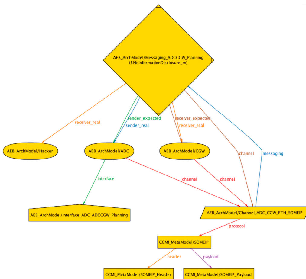
Figure 8. Counterexample of information disclosure attack in AEB system.
