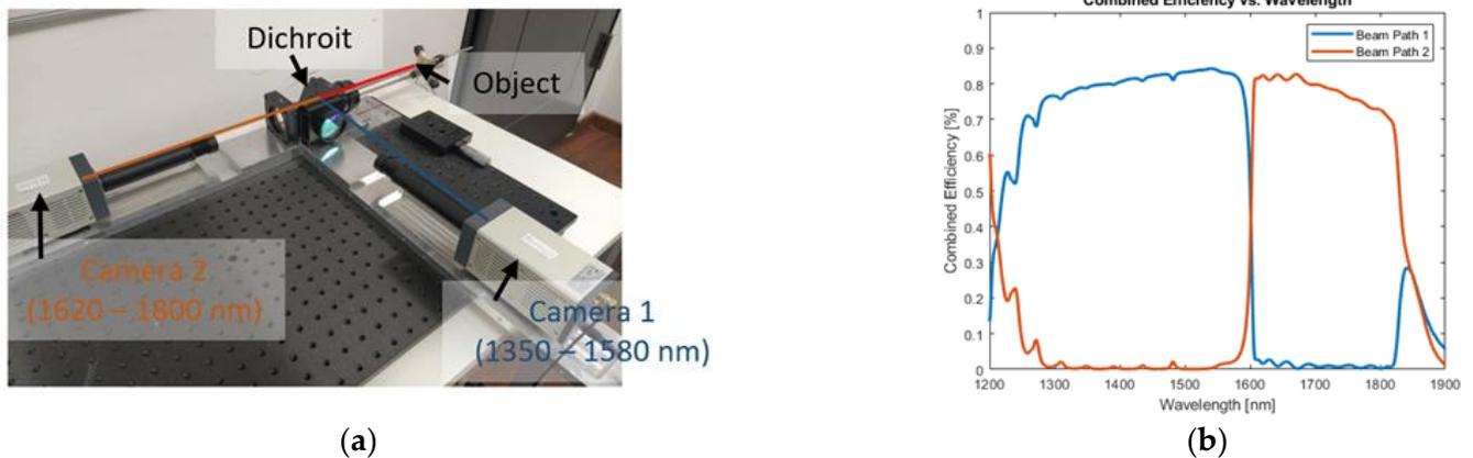
**Figure 1.** (a) Experimental set-up of the two-color-thermography set-up. The system employs two identical but spectrally differently filtered InGaAs-sensor modules (C15370-01, Hamamatsu Photonics Deutschland GmbH, Herrsching, Germany). (b) Simulated combined efficiency along the two spectral differently filtered beam paths (blue: beam path 1 (spectral band: 1350–1580 nm), red: beam path 2 (spectral band: 1620–1800 nm)) plotted against the wavelength.
