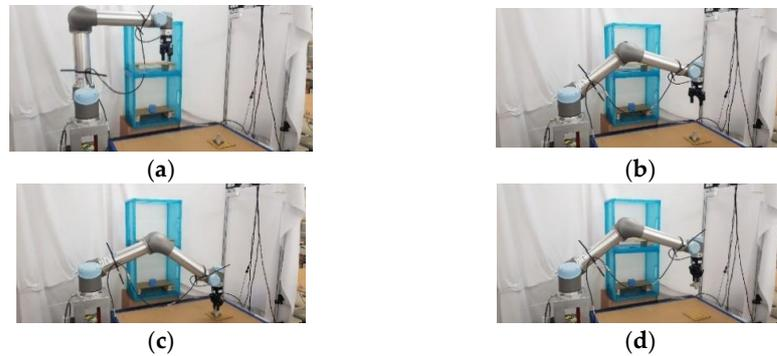
**Figure 17.** Snapshot of the robot manipulator during the object pick-and-place in Task 1. (a) Initial position. (b) Move to the top of Object A. (c) Move downward to grasp Object A. (d) Move upward to the top of the table.
