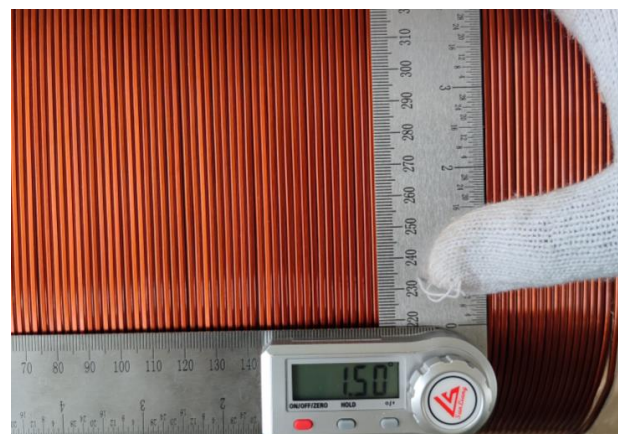
Figure 3. Manual measurement of winding tilt angle.
