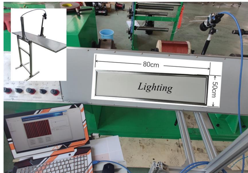
Figure 28. Winding equipment and image capture device.
