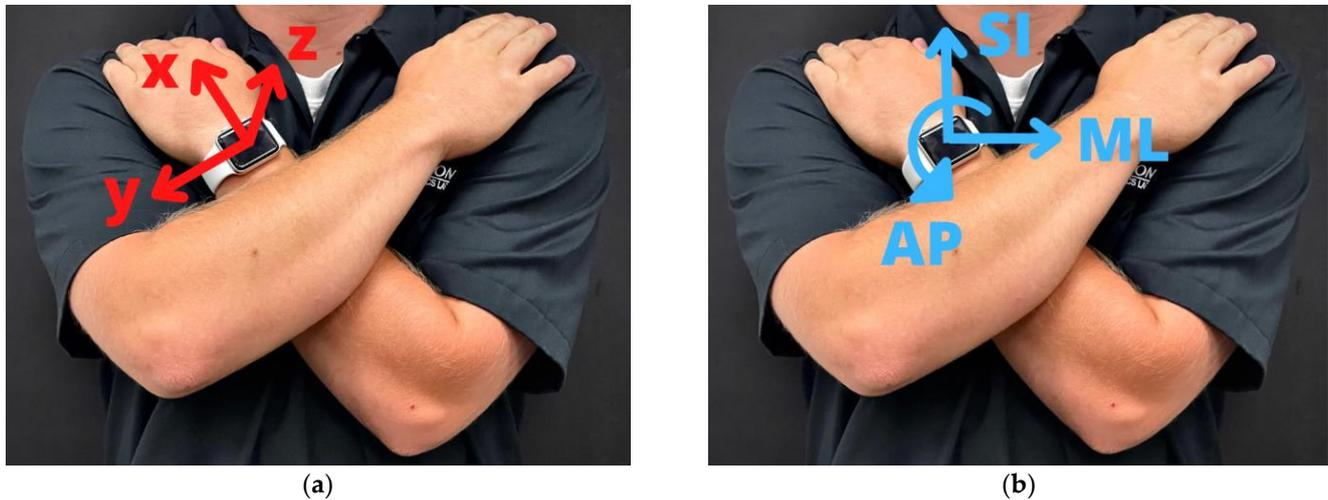
**Figure 1.** (a) Smartwatch's inertial coordinate system, showing the directions in which the smartwatch records acceleration, rotation rate, and gravitational field. (b) Global coordinate system, which contains the anterior-posterior (AP) direction, mediolateral direction (ML), and superior-inferior (SI) direction.
