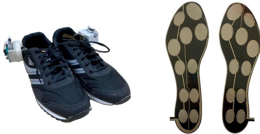
**Figure 1.** Instrumental shoes with inertial sensing and foot pressure measurements at the big toe, little toe, metatarsus (medial, middle, lateral), arches (medial, lateral), fore heels (medial, lateral), and heels (medial, lateral).
