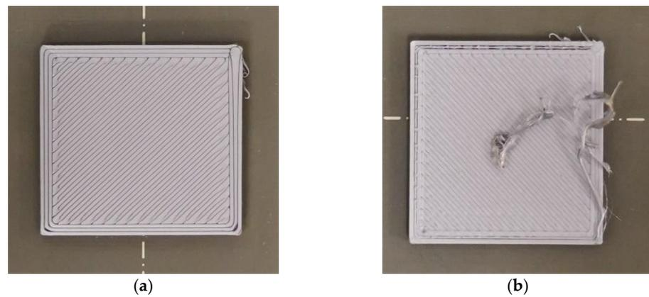
**Figure 1.** Photographs of (a) nondefective and (b) defective samples.
