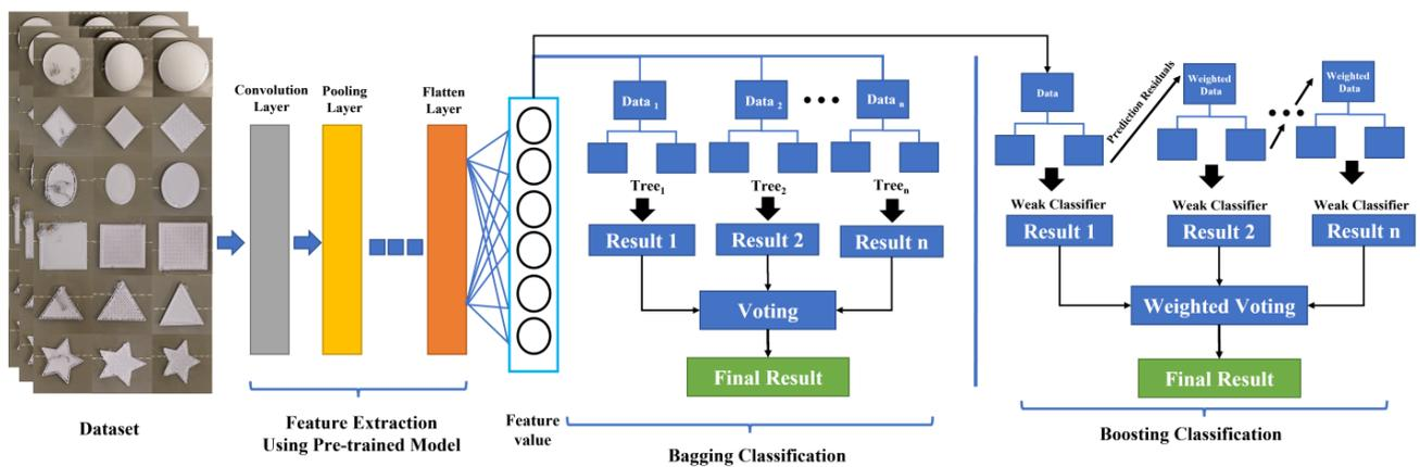
**Figure 4.** The flow graph of the proposed method for bagging or boosting classification.
