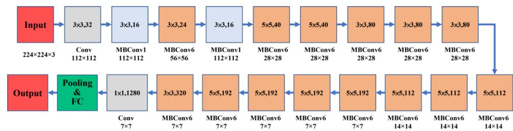
Figure 9. EfficientNetB0 architecture.
