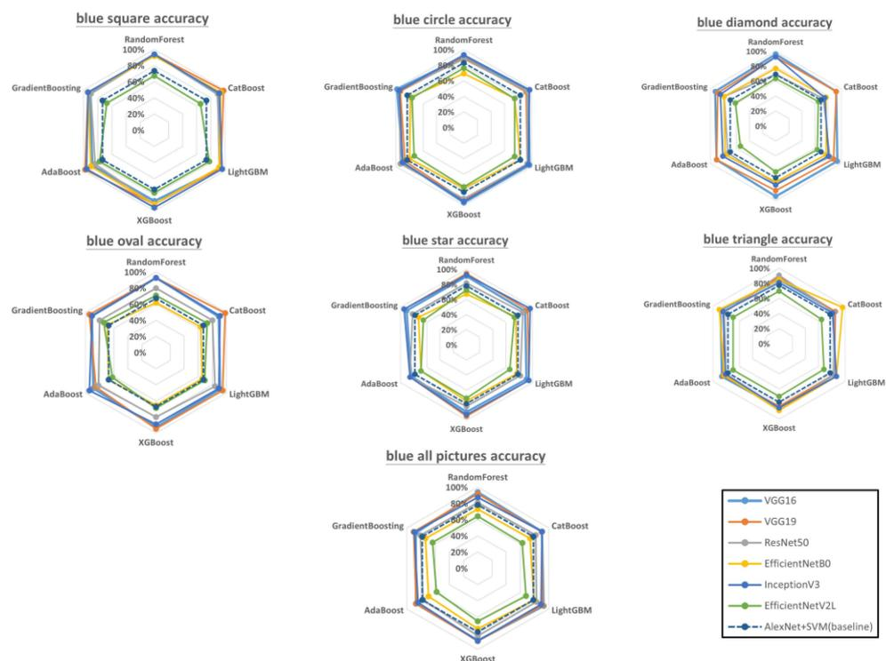
**Figure 12.** Accuracy of each model combination for blue-colored geometries (raw data are presented in Appendix C). The dotted regular hexagon is the baseline using AlexNet with SVM.
