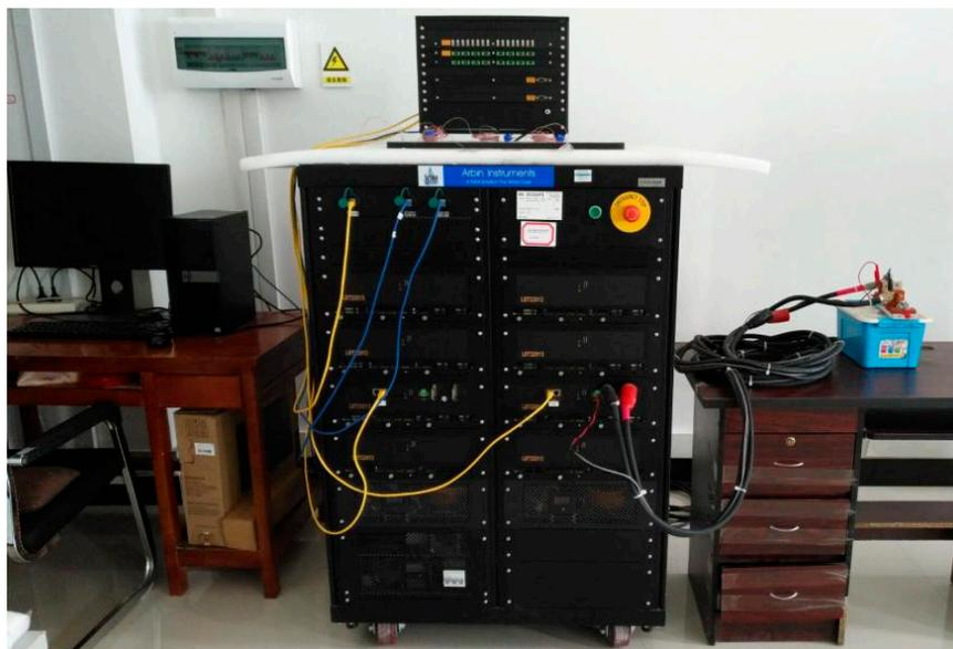
**Figure 2.** Arbin test rig and NCM532 lithium-ion batteries.
