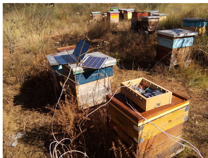
Figure 2. Monitor system setup, installation of the microphones in five bee colonies of the apiary located in Zacatecas, México.
