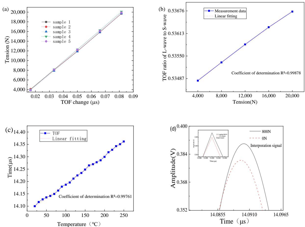
**Figure 7.** (a) Relationship between the TOF difference and the tension; (b) TOF ratio of the first longitudinal wave to the first shear wave as a function of the tension; (c) relationship between the temperature and TOF in an unstressed bolt; (d) TOF change before and after the applied axial preload of 800 N after interpolation. The inset is the original temporal signal of the first longitudinal wave for the cases of 0 N and 800 N.
