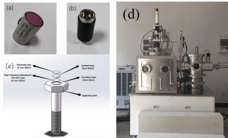
**Figure 2.** Photographs of (a) a commercial piezoelectric probe of 10 MHz and (b) a magnetically mounted transducer connector; (c) schematic diagram of a high-frequency M8 smart nickel-based superalloy bolt; (d) photograph of radio frequency magnetron sputtering.
