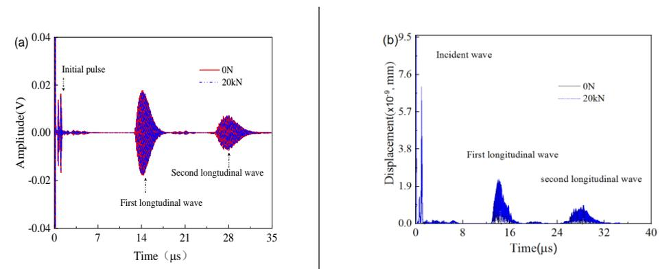
**Figure 4.** (a) The simulated temporal ultrasonic signal inside the nickel–based superalloy bolt, (b) displacement field contrast of the upper surface between the bolt with 20 kN axial preload applied and the slack bolt.
