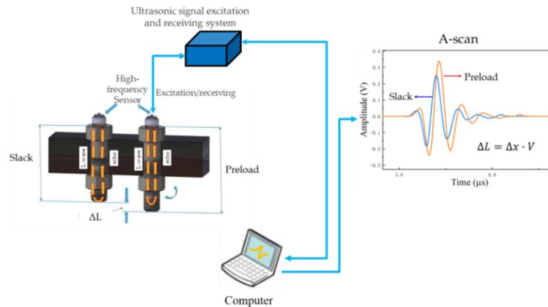
**Figure 1.** Experimental setup schematic and fundamental principle diagram of measuring bolt axial preload by the mono-wave method. (L-wave: longitudinal wave,  $V$ : velocity of longitudinal wave,  $\Delta L$ ,  $\Delta x$ : length and time change of the smart bolt induced by the preload compared with the slack bolt).
