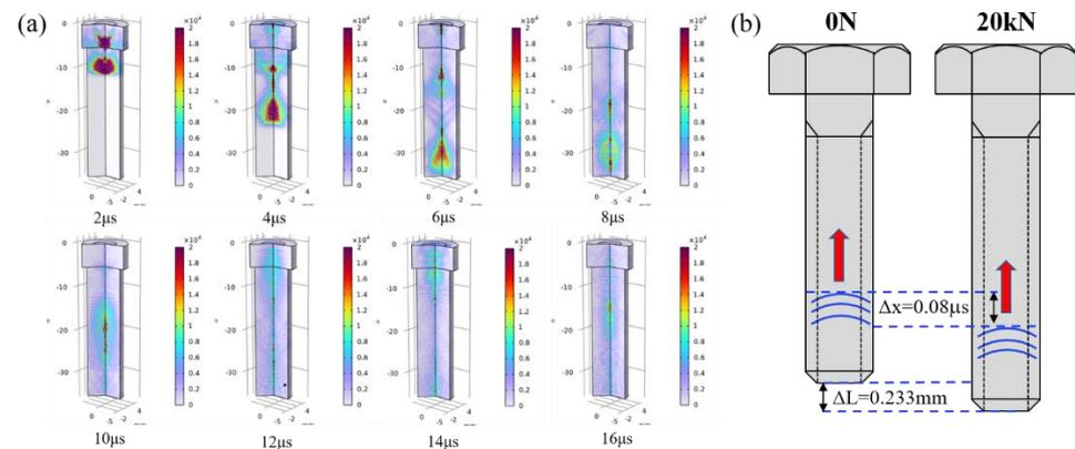
**Figure 3.** (a) Evolution of the ultrasonic wave inside the nickel–based superalloy bolt, (b) schematic diagram of ultrasonic wave propagation difference between the slack bolt and the bolt with 20 kN applied.
