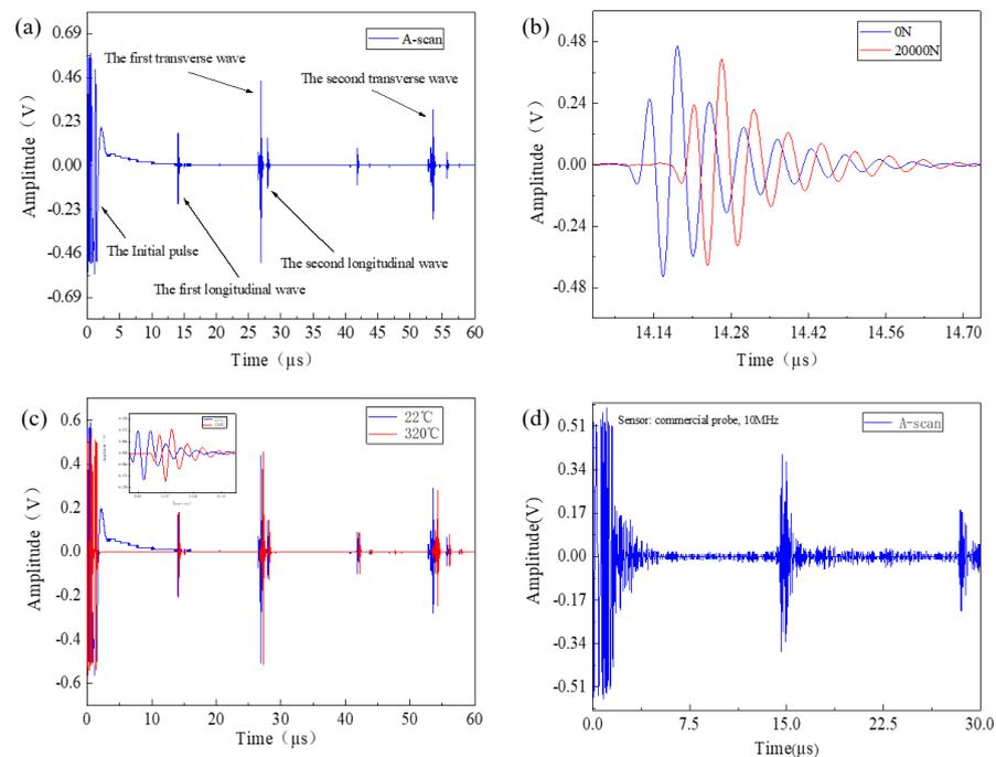
**Figure 5.** (a) The measured A-scan waveform collected from the high-frequency, piezoelectric thin-film sensor, (b) comparing TOF change of the pulse echo before and after applying tension at 20 kN, (c) A-scan waveforms of the smart bolt at 22 °C and 320 °C (the insert compares the waveform of the first longitudinal wave for the bolt at 22 °C and 320 °C), (d) the measured A-scan waveform collected from the commercial piezoelectric probe.
