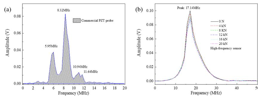
**Figure 6.** Frequency spectra of the measured ultrasonic wave collected from (a) the commercial PZT probe and (b) the high-frequency piezoelectric sensor.
