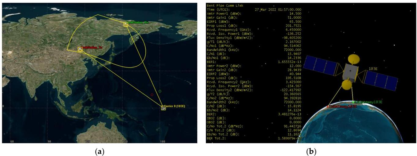
**Figure 7.** Scenario 1 operation (a) 183° E bent pipe transponder operation (b) Bent pipe of Yamal 183E transponder composite link calculation.
