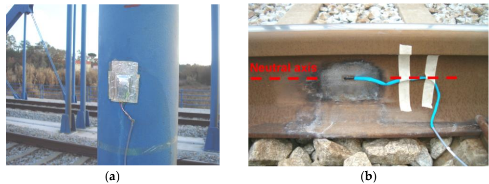
Figure 14. Strain measurement: (a) hanger P3; (b) rail.
