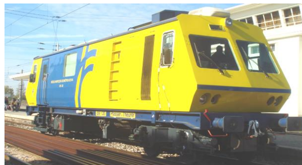
Figure 4. Track inspection vehicle EM 120 from IP.
