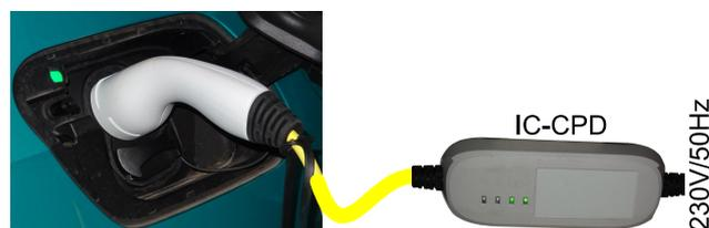
**Figure 2.** The photo of the connector in electric vehicle (during charging) and the charging current controller (IC-CPD).
