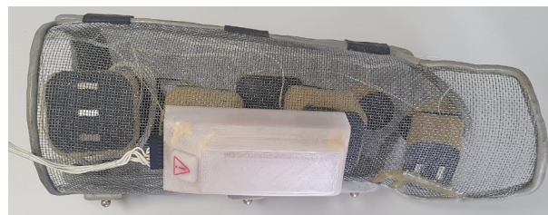
Figure 8. Orthosis with the electrodes and the STIMGRASP stimulator.
