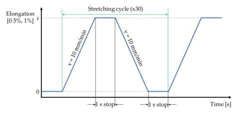
Figure 2. Stretching cycle of NiTi wire.
