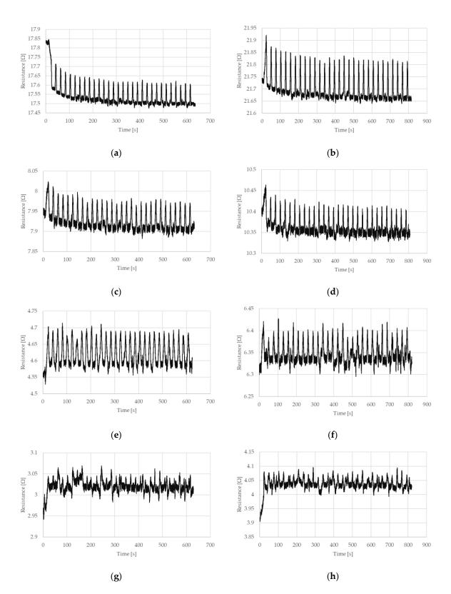
**Figure 5.** Resistance of NiTi wires recorded during cyclic stretching, in which the stretching strain is 1% and (**a**) the diameter,  $D = 100 \mu m$  and the length, L = 150 mm, (**b**)  $D = 100 \mu m$  and L = 200 mm, (**c**)  $D = 150 \mu m$  and L = 150 mm, (**d**)  $D = 150 \mu m$  and L = 198 mm, (**e**)  $D = 200 \mu m$  and L = 148 mm, (**f**)  $D = 200 \mu m$  and L = 200 mm, (**g**)  $D = 250 \mu m$  and L = 149 mm, and (**h**)  $D = 250 \mu m$  and L = 200 mm.
