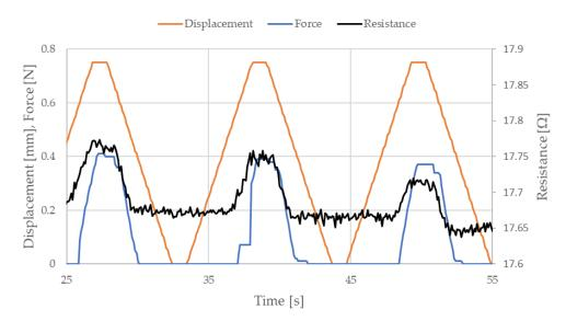
**Figure 6.** Selected parts of the measured data for cyclic stretching of a NiTi wire with diameter 100 µm and length 150 mm, where the strain is 0.5%.
