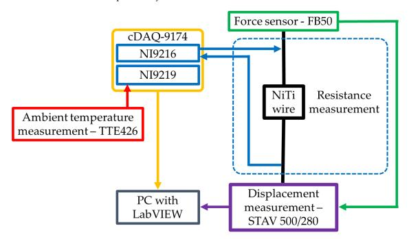
Figure 3. Schematic for the test stand.
