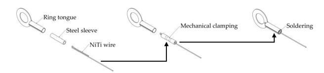
Figure 1. Stages for the creation of the NiTi wire fastening.
