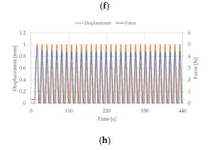
**Figure A1.** Force and deformation recorded during cyclic stretching of NiTi wires where stretching strain was 0.5%: (**a**)  $D = 100 \mu m$ , L = 150 mm; (**b**)  $D = 100 \mu m$ , L = 200 mm; (**c**)  $D = 150 \mu m$ , L = 150 mm; (**d**)  $D = 150 \mu m$ , L = 198 mm; (**e**)  $D = 200 \mu m$ , L = 148 mm; (**f**)  $D = 200 \mu m$ , L = 200 mm; (**g**)  $D = 250 \mu m$ , L = 149 mm; (**h**)  $D = 250 \mu m$ , L = 200 mm.
