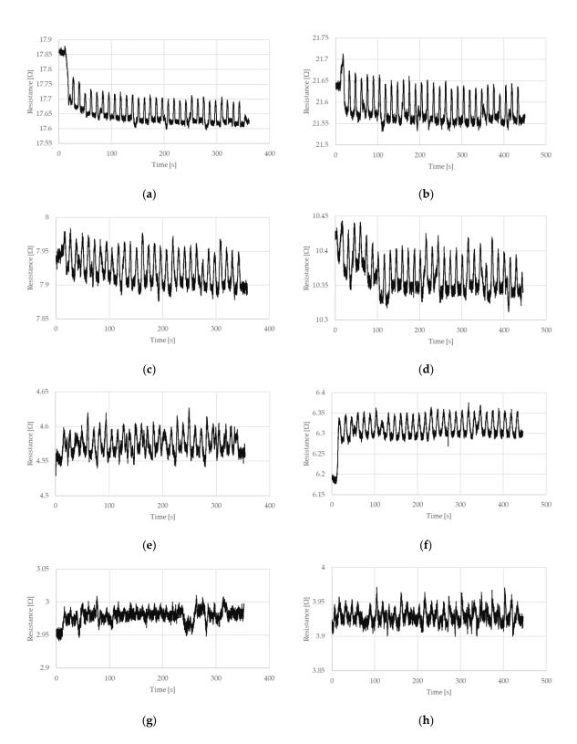
**Figure 4.** Resistance of NiTi wires recorded during cyclic stretching, in which the stretching strain is 0.5% and (**a**) the diameter, D = 100  $\mu$ m and the length, L = 150 mm, (**b**) D = 100  $\mu$ m and L = 200 mm, (**c**) D = 150  $\mu$ m and L = 150 mm, (**d**) D = 150  $\mu$ m and L = 198 mm, (**e**) D = 200  $\mu$ m and L = 148 mm, (**f**) D = 200  $\mu$ m and L = 200 mm, (**g**) D = 250  $\mu$ m and L = 149 mm, and (**h**) D = 250  $\mu$ m and L = 200 mm.
