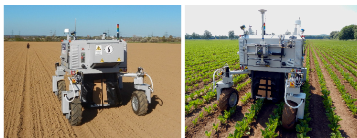
Figure 2. Field robot BoniRob [78].
